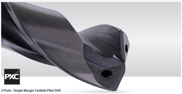
The PXC Series is a multi-purpose Pilot Drill designed to be used before a long-drill begins perforation. Its design includes a 30° helix and 140° point geometry, for superior drill penetration and accuracy. Furthermore, the PXC Series has internal coolant holes that allow for improved operating temperatures, at increased speeds and feeds.
